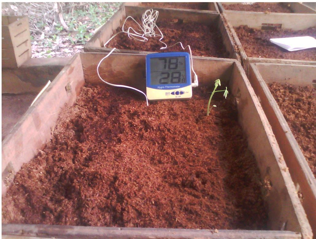
**Figure 2. Thermo-hygrometers indicating the RH and Temperature**
