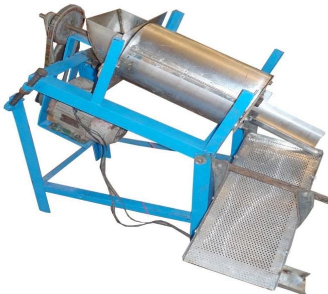
**Plate 1: Custard apple de-pulping machine developed by Bakane et al. (2015)**
