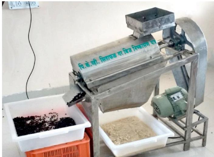
**Plate 2: Custard apple de-pulping machine developed by Nambi et al. (2017)**
