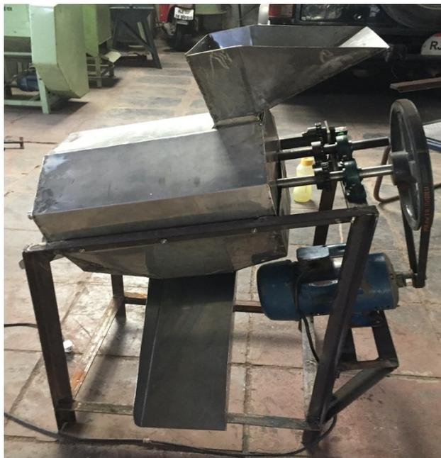
**Plate 3: Custard apple de-pulping machine developed by Mudgal (2020)**
