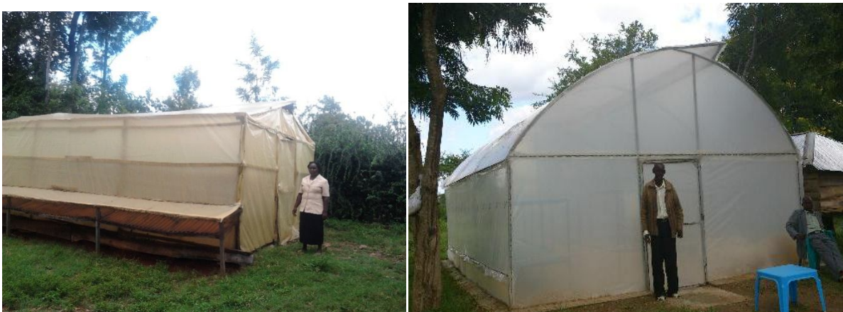
Figure 2. Types of solar dryers (left: gable roof dryer; right: parabolic or semi-circular shape).
