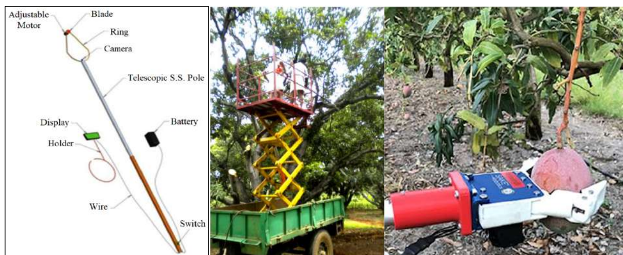
Figure 3: (a) Battery-operated handheld harvesting device (Jhala, et al., 2018), (b) Tractor-operated hydraulic platform developed by ICAR-IIHR, and (c) The world's first automated mango picking invented by Central Queensland University
