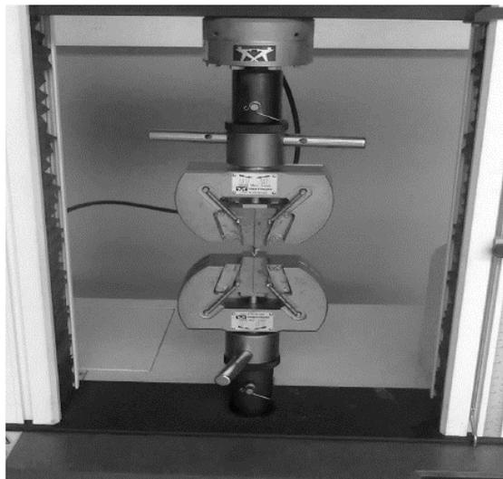
**Figure 3. The Instron Universal Testing Machine (Model 3369) showing a rectangular strip of roselle calyx being pulled axially for determination of tensile properties**
